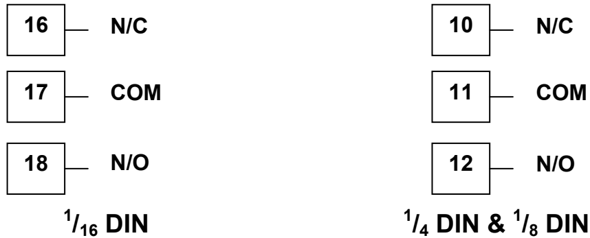
Figure 27. Option Slot 3 - Relay Module
