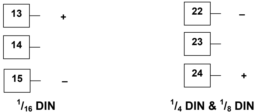
Figure 26. Option Slot 2 - Linear Voltage & mADC module
