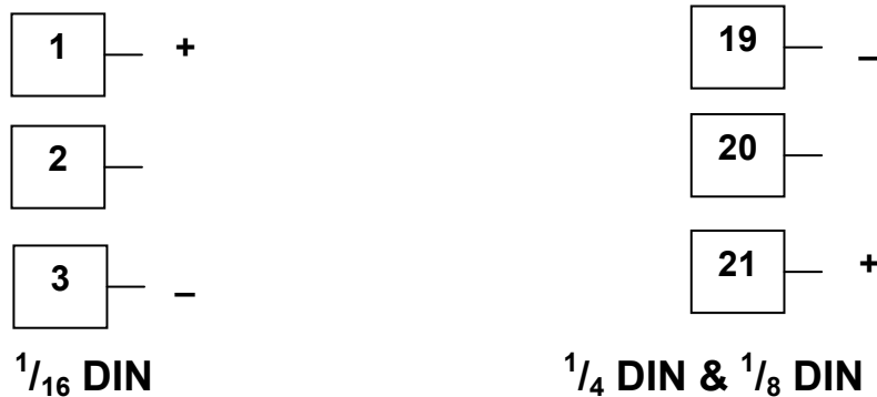
Figure 19. Option Slot 1 - SSR Driver Module
