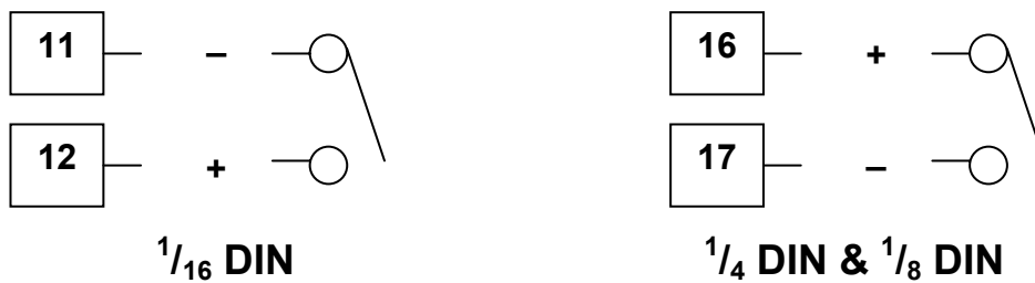
Figure 33. Option Slot A – Digital Input Module
