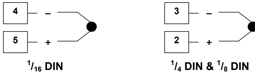
Figure 15. Thermocouple Input Connections
