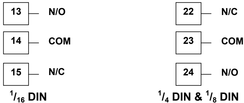
Figure 22. Option Slot 2 - Relay Module
