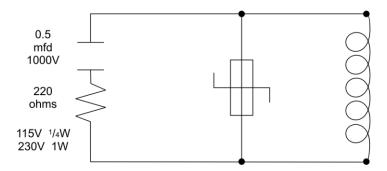
**Contacts:** - Arcing may occur across contacts when they open and close. This results in electrical noise as well as damage to the contacts. Connecting a properly sized RC network can eliminate this arcing.
