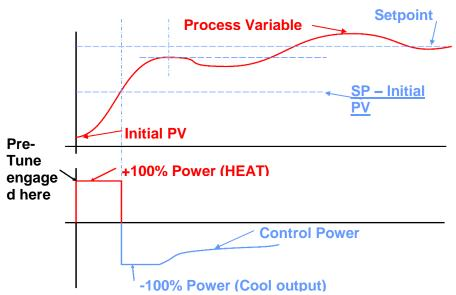
application has been changed. It will automatically disengage once complete. Ideally the Tune program should be used when the load temperature is at or near ambient. Care should be taken to ensure that any overshoot is safe for the process and if necessary tune at a lower setpoint.
