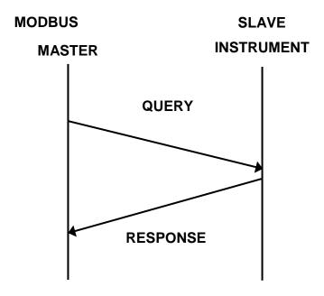
A message for either a QUERY or RESPONSE is made up of an inter-message gap followed by a sequence of data characters. The inter-message gap is at least 3.5 data character times - the transmitter must not start transmission until 3 character times have elapsed since reception of the last character in a message, and must release the transmission line within 3 character times of the last character in a message.
