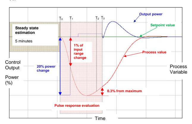
The process will reach a maximum excursion away from the setpoint and then return towards the setpoint. After a 0.3% recovery from maximum excursion, the pulse response characteristics are used to calculate the correct tuning terms.
