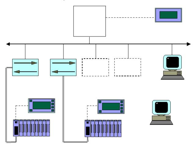
The MLC 9000 RS485 ports are connected to the PROFIBUS system via Gateways. These convert the PROFIBUS protocol to MODBUS for use by the MLC 9000. The Gateways are slave devices on the main bus, but acts as masters for the RS485 MODBUS connections to the MLC 9000 attached to them.
