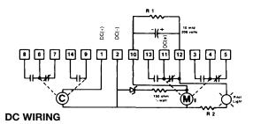
**CAUTION!:** Power for motor must be jumped from Terminal 1 to 11. Do **NOT** apply power to Terminal 12.
