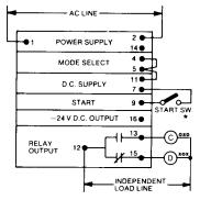
REPEAT CYCLE PULSE GENERATOR — Uninterrupted start signal
