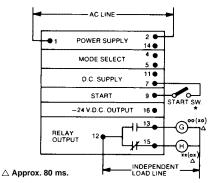
\*Start switch must be closed — or DC start signal must be **on** — for entire cycle. Timer resets when start switch opens or DC start signal turns **off**. to start form DC voltage, apply external ground on 11 and start signal on 9.
