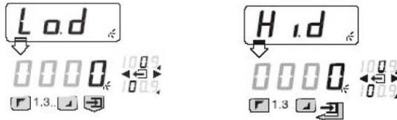
When “Lod” appears, press key to toggle to proper digit. Use the and keys to select desired value. Repeat procedure until all digits have been set, press to confirm and advance to the next step, “Hid”. Repeat the same procedure to select and confirm the “Hid” values. Press to confirm. Press to advance to the next program step sequence.
