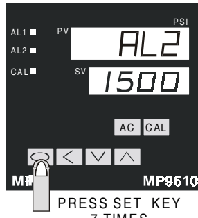
PRESS LEFT UP AND DOWN KEY TO CHANGE ALARM POINT
