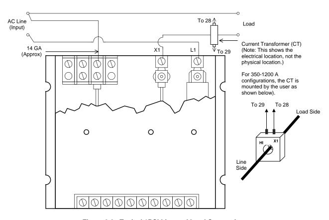
Figure 2-3. Typical 1PCI Line and Load Connections
