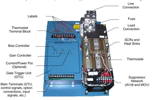
Figure 1-2. Key Hardware Components of a Typical 1PCI Series Power Controller
