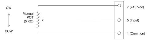
Figure 2-5. Remote Control with a Potentiometer
