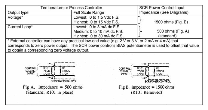
As an example of the use of Table 3-1, consider a typical controller that will supply 10 V maximum for a 0-20 mA current loop. According to Table 3-1, a controller impedance of 5000hm would be correct for proper operation, and the external 7500hm resistor would not need to be removed.
