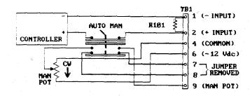
Figure 3-3. Auto/Man Control with Controller and Remote Potentiometer
