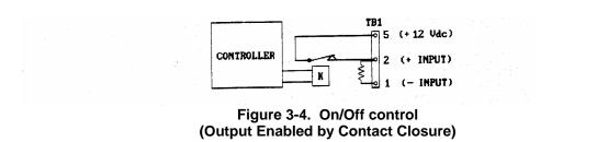
Calibrate the system by performing the steps in 3-2. Note that zero power demand is accomplished by opening the contacts with the controller, and maximum power demand is present when the contacts are closed.
