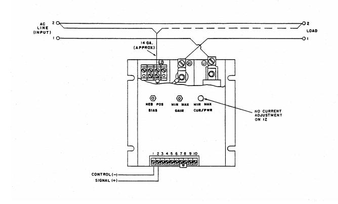
Figure 2-1. Typical 1Z Line and Load Connections
