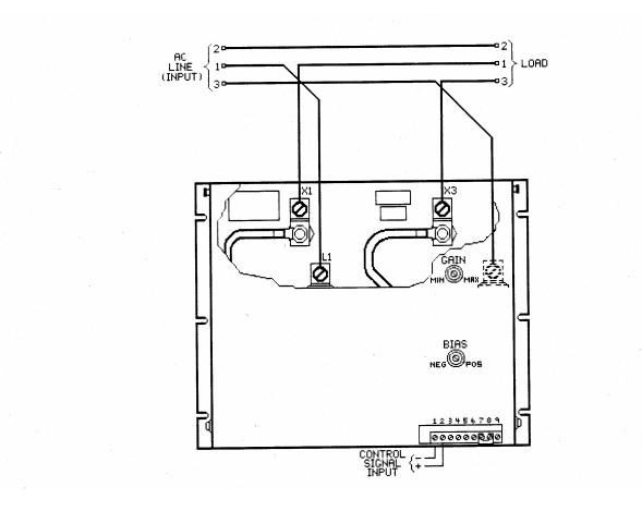
Figure 2-1. Typical 2Z Line and Load Connections
