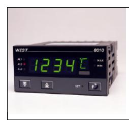
The West 8010 is a 1/8 DIN microprocessor based digital indicator. Available with red or green displays. One latchable relay is fitted as standard, plug-in modules allow two more alarm relays, PV retransmission or transmitter PSU.
